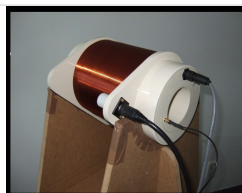
Earth's Field MRI apparatus — NMR coil assembly
