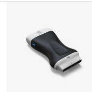
Clarius handheld ultrasound transducer (L15/C3 series)
